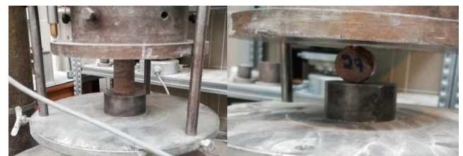
Figure 2. Uniaxial compressive test and Brazilian strength test
