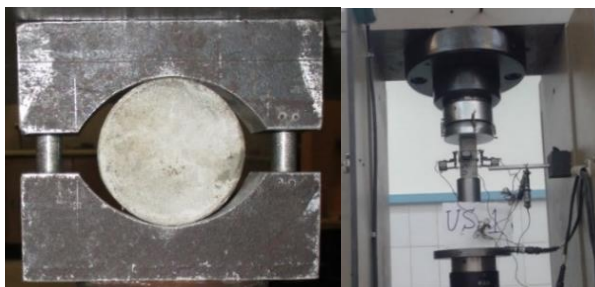
Fig.1. Experimental tests: Brazilian test, UCS test.
