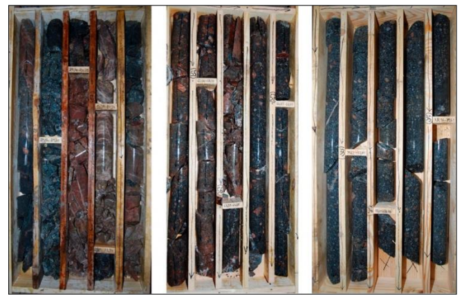
Figure 3. Rock cores with different fracture density of the Mórággy Granite Formation.
