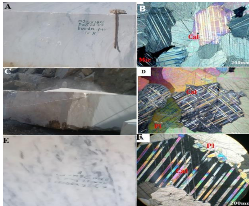
Fig. 9. A, C & E field photographs of marble exposures and B, D & F marble thin section under XPL (where Cal: - Calcite; Mic:- Microcline, and Pl:- Plagioclase).
