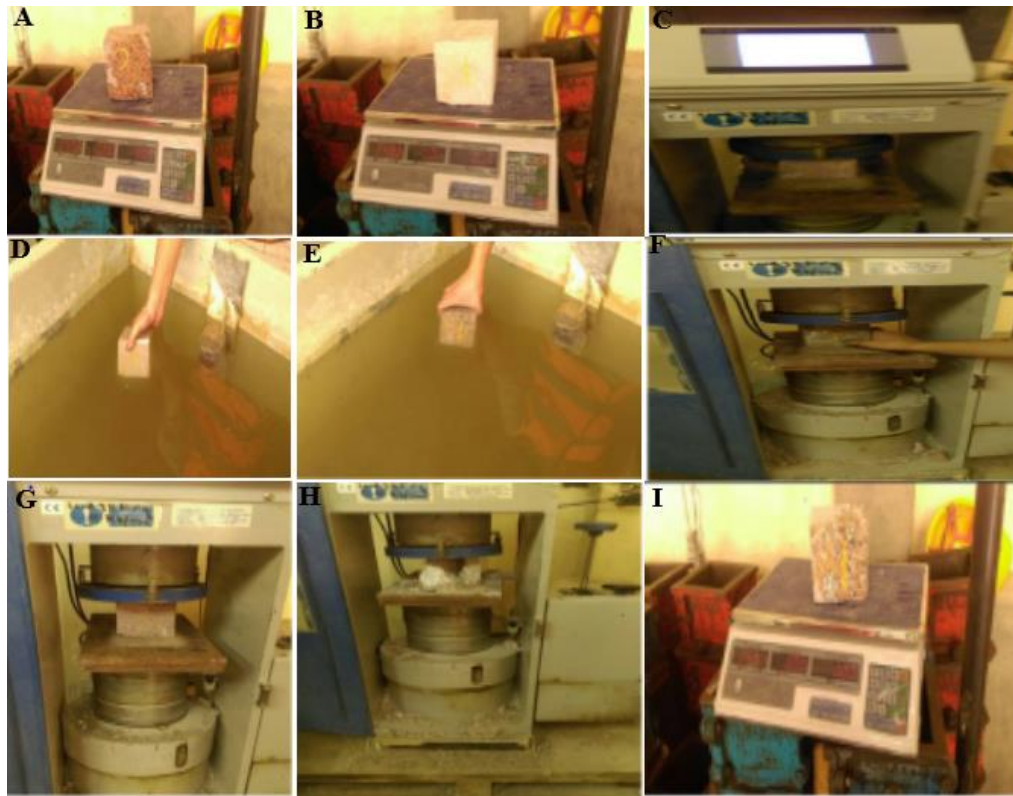
Fig. 6. Photographs showing the dry density test of granite (A&I) and marble (B), water absorption test for marble (D) and granite (E), and compressive strength test for granite (F&G) and marble (C&H).
