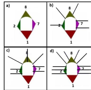
Fig. 12. 2D distribution of support units across the excavation with different support spacing (a) no support unit installed, (b) 2.0m x 2.0m (c) 1.5m x 1.5 (d) 1.0m x 1.0m
