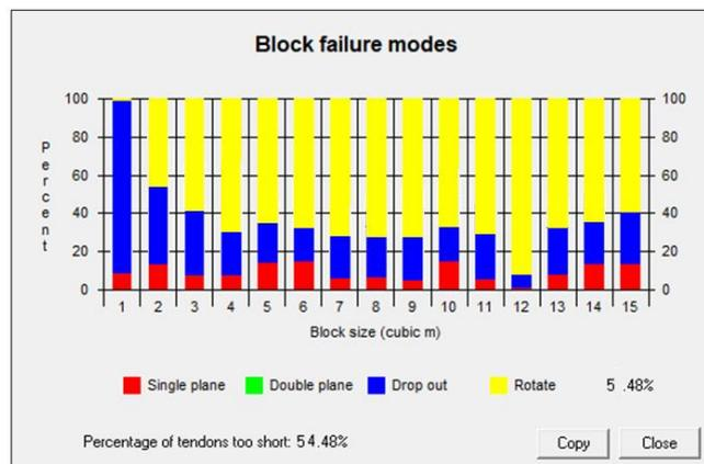
Fig.9. Block failure modes.
