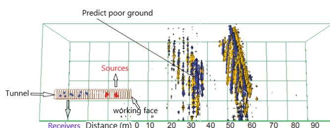
**Fig. 2.** Side view of TRT detection results at 40m in North direction level 7
