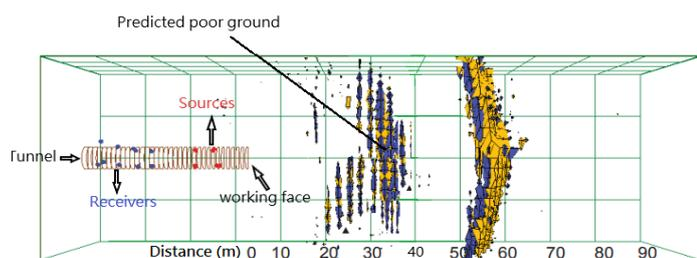
**Fig. 1.** Top view of TRT detection results at 40m in North direction level 7
