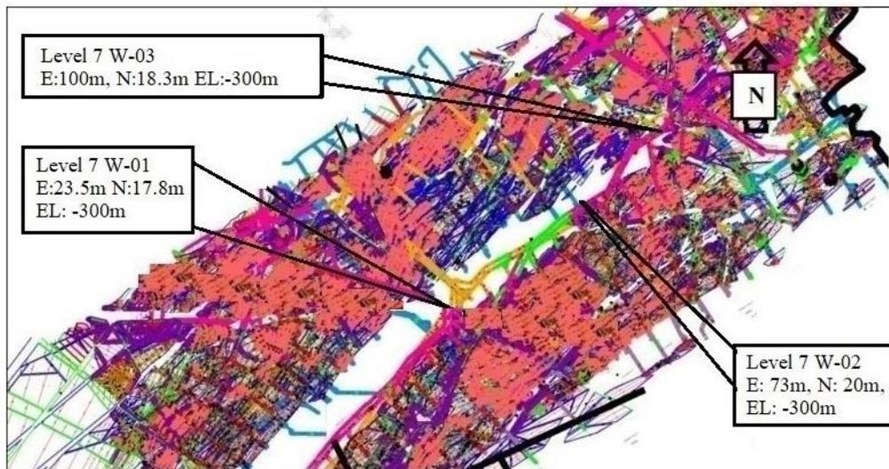
Fig. 5. Three district areas (W-01, W-02, and W-03) indicating level 7 borehole locations (the Gold Mine Geotechnical Database).
