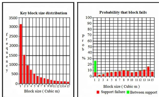
Fig. 8. Key block size distribution and Probability that block fails
