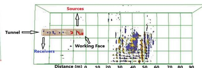
**Fig. 4.** Front view of TRT detection at 160m in North direction at level 7
